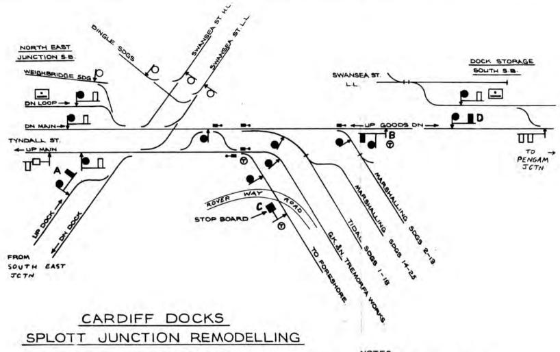
FINAL LAYOUT AND NEW SIGNALLING ARRANGEMENTS.
